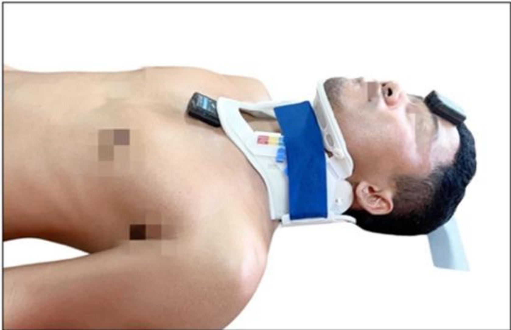
Figure 1: Position for installing inertial measurement unit (IMU) on the forehead and the chest.
